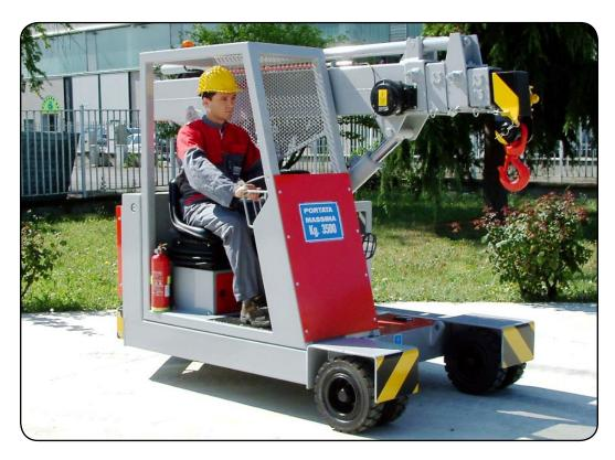
DRIVE: DC 3.3 kW - 24 V fanned reversible electric motor with MOSFET electronic control HF and energy saving, self diagnostic, speed and temperature checks (no. 2 thermostasts), brush wear warning. Foot hydraulically operated brake to drive wheel. Hand brake mechanically operated. Gear box between motor and drive wheel in oil bath. Speed up to 8 km/h.
