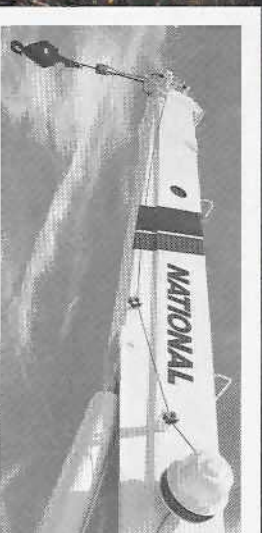
National's anti two block system is standard on all National cranes (as of June 1, 1986). Photos in this brochure taken prior to that date may not show the crane equipped with the current standard anti two block protection system.
