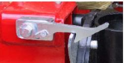
If the loader is equipped with swing-up outrigger legs they must also be secured in position before driving off. Before the vehicle is started, disengage the PTO and turn off the pump.
