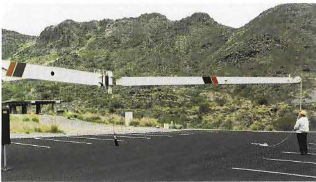
The sequence of photos above shows how the National 1200 29-52 foot jib folds out into a working position.
