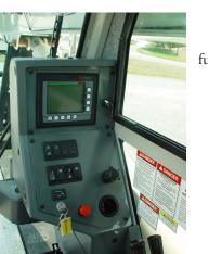
(LMI) is standard on all NBT45 machines. The LCD display is visible in full or low light and displays all crane load lifting values simultaneously. Includes Work Area Definition System (WADS).
