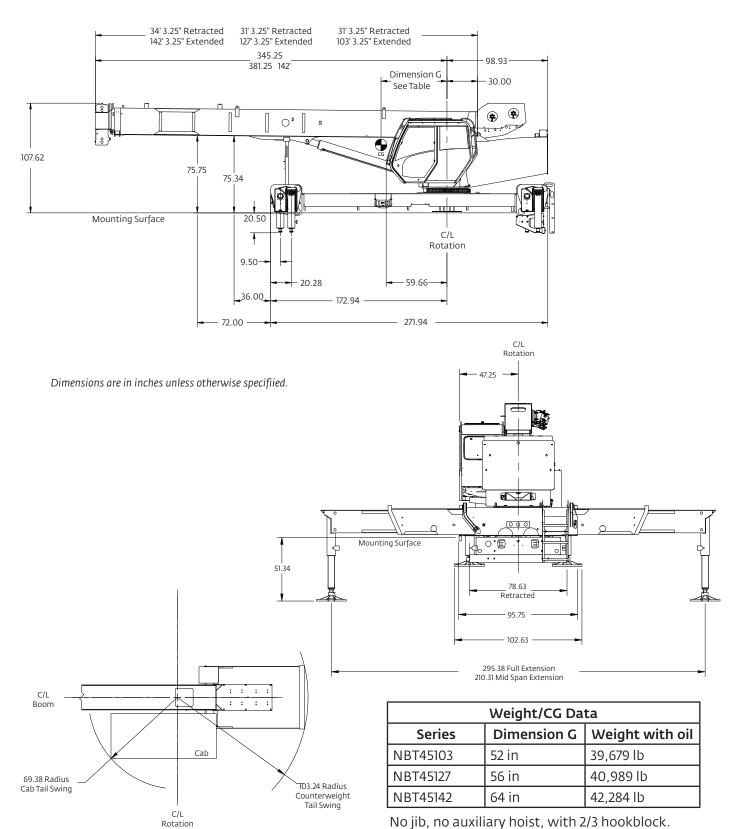
No jib, no auxiliary hoist, with 2/3 hookblock.
