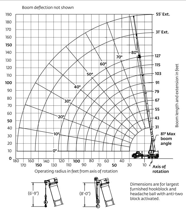
\*Drawing is to show the physical reach of the machine. Always refer to load chart to see what portions of this range are structurally and stability limited.
