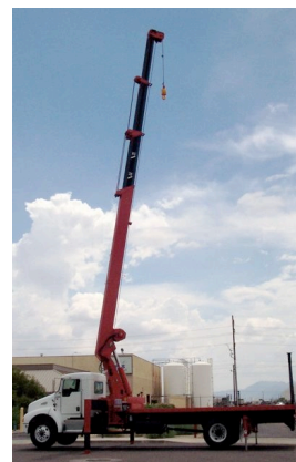
Boom Length 82 ft. - Retracted 25 ft.
