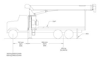
Requires front SFO stabilizer to give machine full capacity 360° around the truck. Truck must meet the minimum requirements above. Front stabilizer gives the machine a solid base, helping the operator control loads precisely. Extended front frame rails required for SFO installation.
