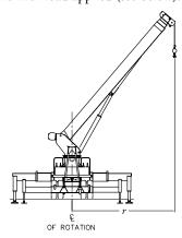
2. Loaded boom angle ( $\angle$ ), as shown in the column headed by  $\angle$ , is the included angle between the horizontal and longitudinal axis of the boom base after lifting rated load at rated radius (see below).
