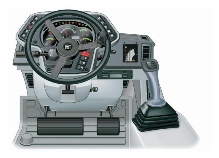
**Intuitive Control Layout.** All day operator comfort and efficiency is ensured through our simple, logical control layout.
