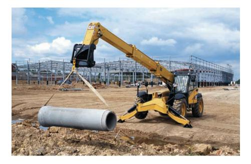
**Quick Coupler.** An IT interface is standard on the B-Series. It is available in both a manual and a hydraulic version.
