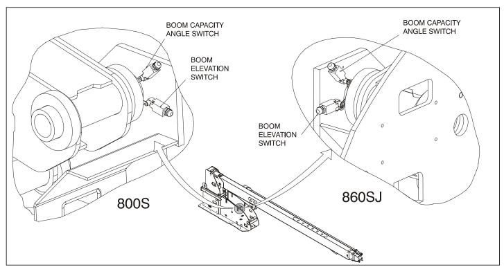
Figure 2-6. Limiting and Cut-Out Switches - Sheet 1 of 2
