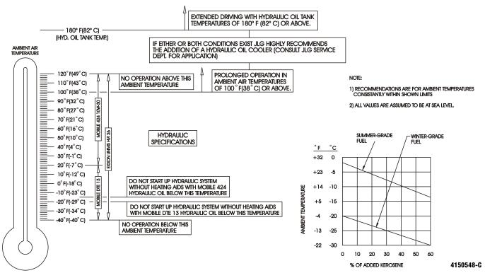
Figure 6-3. Engine Operating Temperature Specifications - Deutz - Sheet 2 of 2
