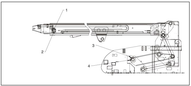
Figure 2-4. Horizontal and Capacity Limit Switches - Sheet 1 of 2
