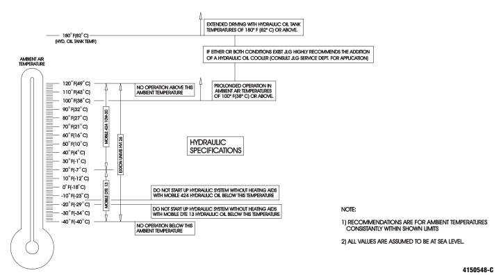
Figure 6-7. Engine Operating Temperature Specifications - Caterpillar - Sheet 2 of 2
