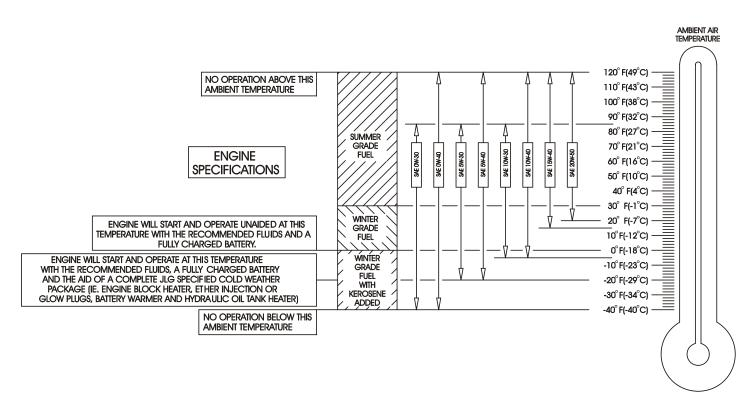
Figure 6-2. Engine Operating Temperature Specifications - Deutz - Sheet 1 of 2
