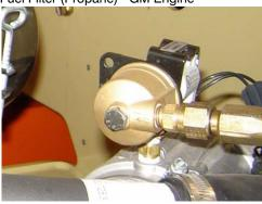
Interval - 3 Months or 150 hours of operation Comments - Replace filter. Refer to Section 6.7, Propane Fuel Filter Replacement
