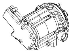
Interval - 3 Months or 150 hours of operation Comments - Drain oil build up. Refer to Section 6.6, Draining Oil Build Up From The Propane Regulator
