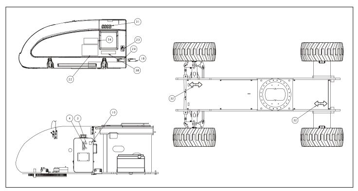
Figure 4-11. Decal Location - Side Entry Platform - Sheet 3 of 5
