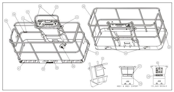
Figure 4-13. Decal Location - Side Entry Platform - Sheet 5 of 5
