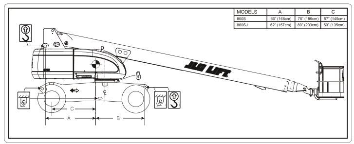
Figure 4-6. Lifting and Tie Down Chart
