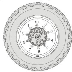
The tightening of the nuts should be done in stages. Following the recommended sequence, tighten nuts per wheel torque chart.
