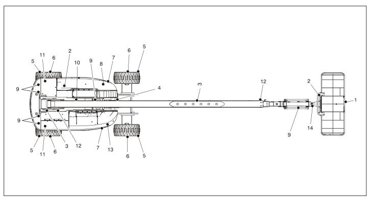
Figure 2-2. Daily Walk-Around Inspection - Sheet 1 of 2
