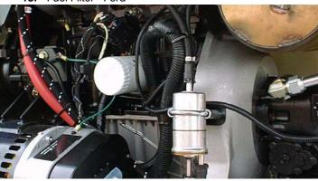
Lube Point(s) - Replaceable Element Interval - Every Year or 1200 hours of operation
