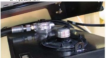
Lube Point(s) - Fill Cap Capacity - 116 liters Tank 124 liters System Lube - HO Interval - Check Level daily; Change every 2 years or 1200 hours of operation.
