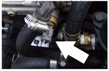
Remove the retainer clip for the LPG fuel temperature sensor and remove the sensor from the regulator body.
