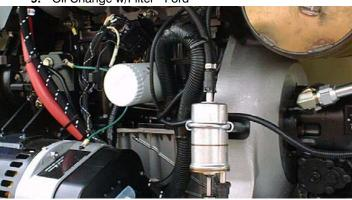
Lube Point(s) - Fill Cap/Spin-on Element (JLG P/N 7014501)
