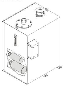
Lube Point(s) - 2 Interval - Every 2 years or 1200 hours of operation, remove and clean at time of hydraulic oil change.
