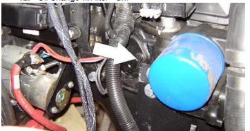
Lube Point(s) - Fill Cap/Spin-on Element (JLG P/N 7027965)
