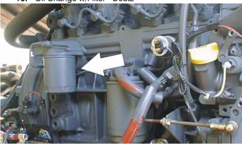
Lube Point(s) - Fill Cap/Spin-on Element (JLG P/N 7016331)
