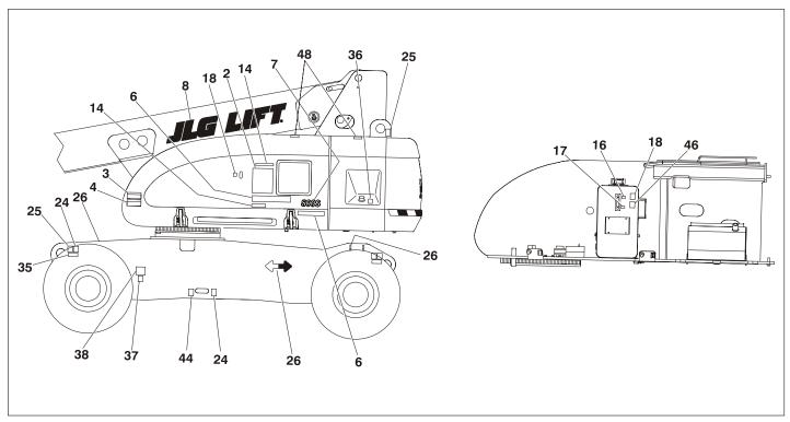
Figure 4-7. Decal Location - Rear Entry Platform - Sheet 1 of 2
