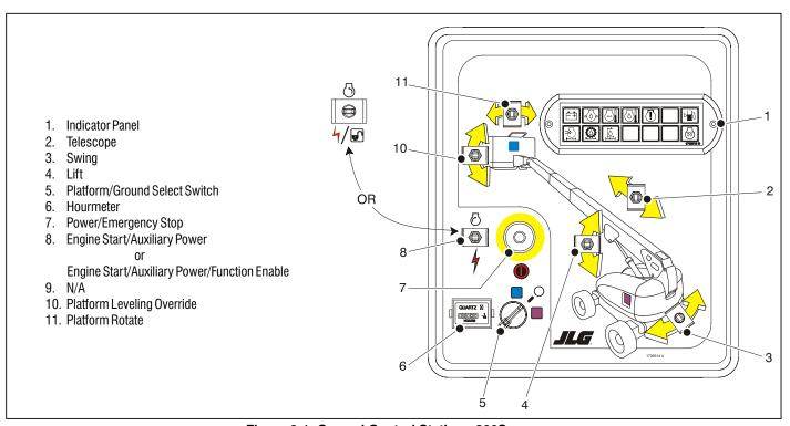
Figure 3-1. Ground Control Station - 800S
