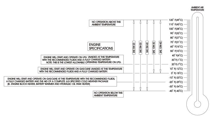
Figure 6-4. Engine Operating Temperature Specifications - Ford - Sheet 1 of 2
