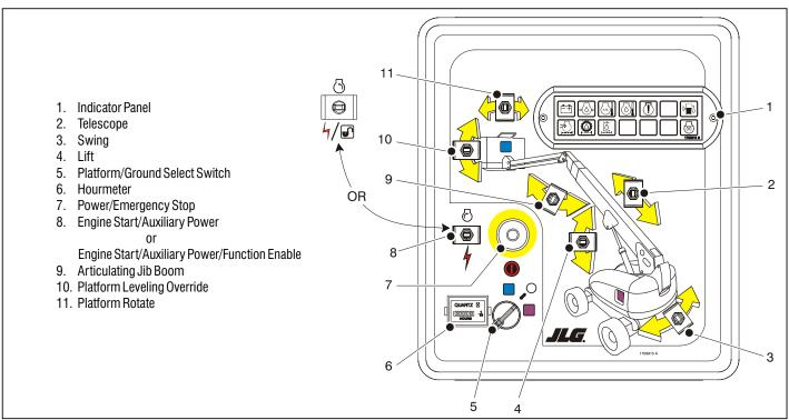
Figure 3-1. Ground Control Station - 860SJ
