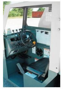
**Cab Standard:** Open air cab shell with overhead safety glass **Optional:** Closed cab with hinged door, heater/defroster, and all window glass
