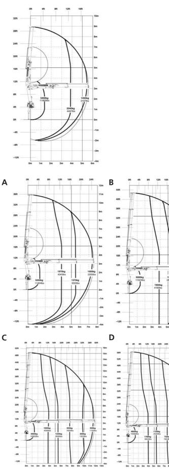
The outreaches stated are with a boom angle of  $20^\circ$  and are therefore not the maximum.
