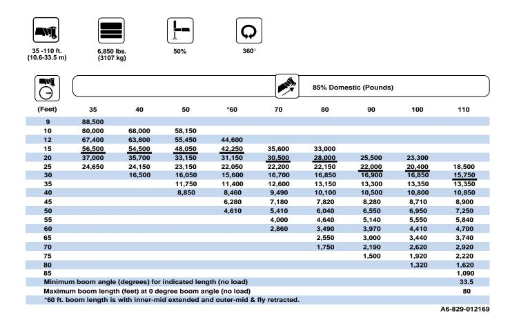
THIS CHART IS ONLY A GUIDE AND SHOULD NOT BE USED TO OPERATE THE CRANE. The individual crane's load chart, operating instructions and other instructional plates must be read and understood prior to operating the crane.
