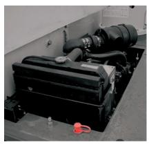
Standard: Cummins QSB 3.3L turbocharged diesel rated @ 99 bhp (73.8kW) @ 2600 rpm.
