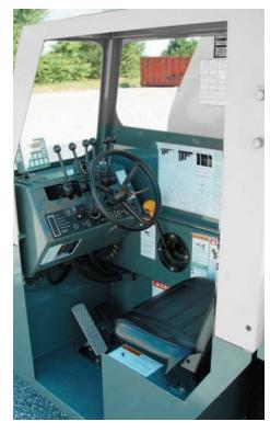
Standard: Open air cab shell w/overhead safety
