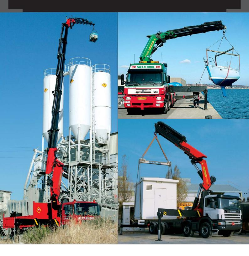
LOW WEIGHT THROUGH USE OF HIGH-STRENGTH FINE-GRAINED STRUCTURAL STEEL
