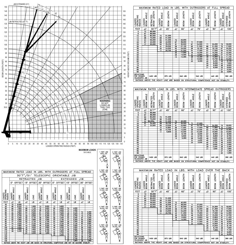
NOTE: Deductions must be made from rated loads for lifting accessories: Fixed jibs, telescopic jibs, overhaul balls, load hooks, snatch blocks and load blocks
