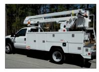
As part of the insulated product line, this versatile ETO model comes with working heights from 35 feet to 42 feet in an articulating, over-center aerial. The ETO 30/33/37 offers continuous rotation, full pressure hydraulic controls, and a positive chain and rod leveling system as standard on its units. A welcome safety feature is also standard and includes internally mounted holding valves that lock cylinders in place in the event of a hydraulic failure. This
