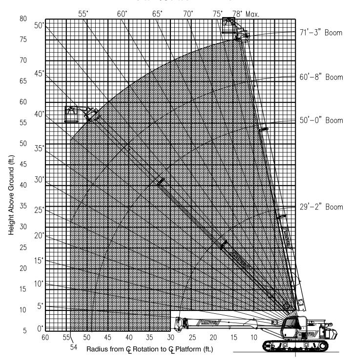
Limits of operation: Maximum load capacity = 750 lb Maximum radius when mounted on main boom = 54 ft
