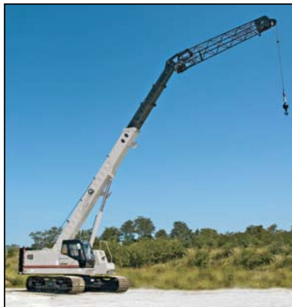
32" grouser track shoes form a wide gauge of 11' 2" (3.40 m) when extended, and 8' 9" (2.66 m) when retracted with two position house lock.
