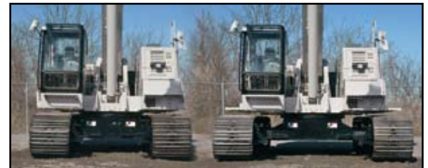
32" grouser track shoes form a wide gauge of 11' 2" (3.40 m) when extended, and 8' 9" (2.66 m) when retracted with two position house lock.
