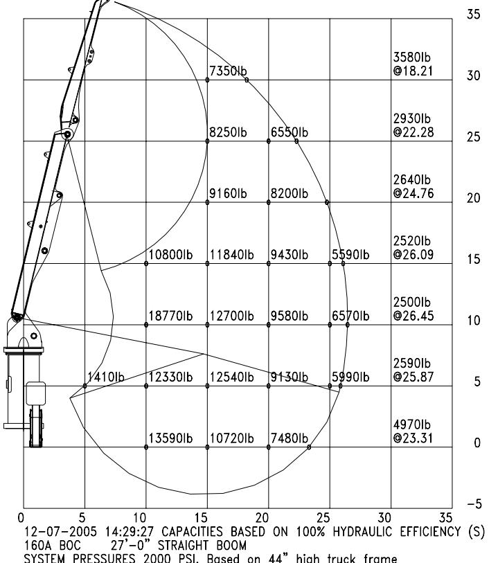
Capacities are based on 100% hydraulic efficiency less attachment.
