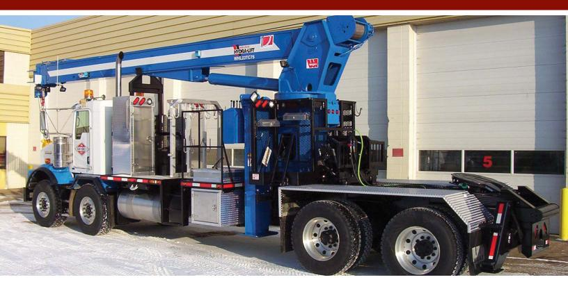
The WHL23TC75 is a mid-capacity crane with a three-stage boom that extends to 75 feet. Introduced in 2004, the model continues to be popular with a wide range of industries that appreciate its durable and rugged design.
