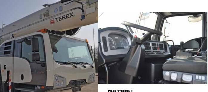
**CRAB STEERING** Possibility for crab steering on left side (door covering) and right side (shift console) of the driver adjustable shift console
