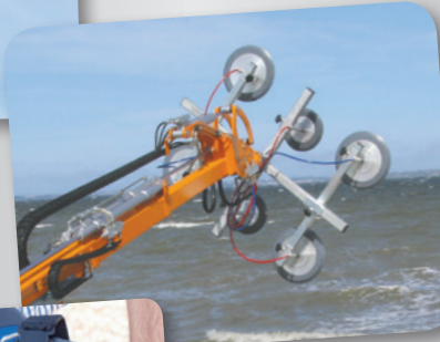
The Smartlift has hydraulic movements in all directions
