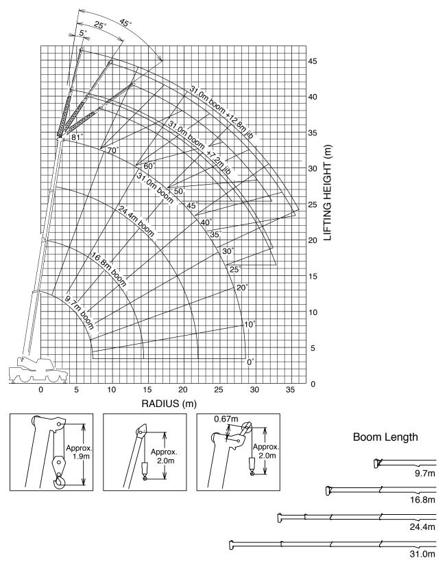
NOTE: The above lifting height and boom angle are based on a straight (unladen) boom, and allowance should be made for boom deflection obtained under laden conditions.
