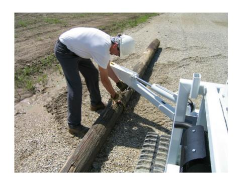
Attach the provided lifting chains to the pole and to the drings on the EZ Hauler 2500 outrigger arms as shown.
