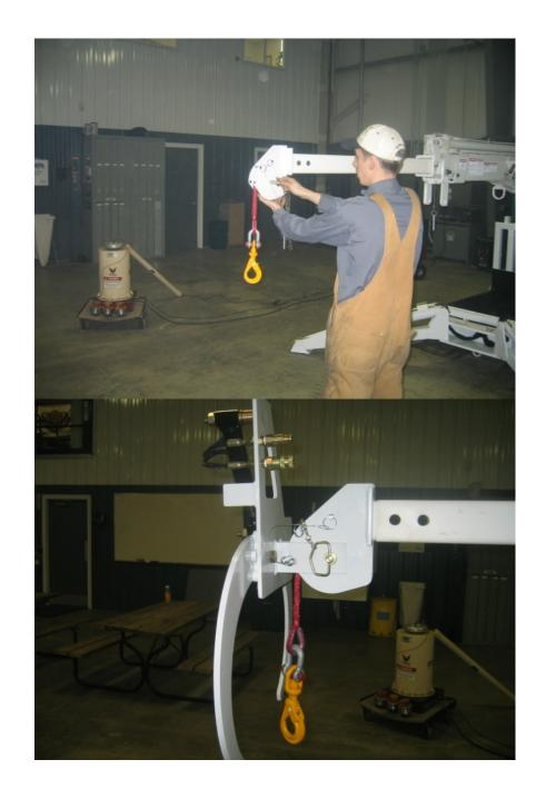
3. Connect hose reel lines to hydraulic claw quick couplers.
