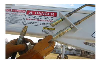
4. Clean the surface of the auger hose and the couplers on the boom. Then attach the auger hose couplers
