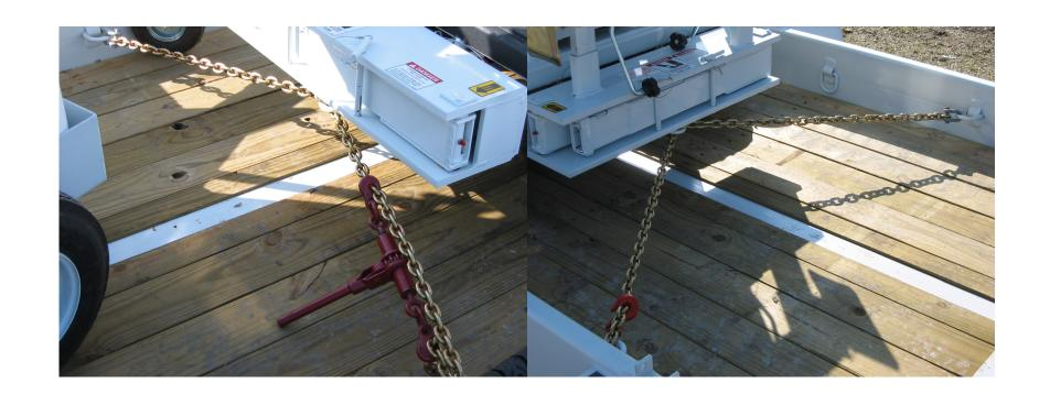
NOTE: The EZ Hauler 2500 is secured for transport at the front and back of the trailer.
