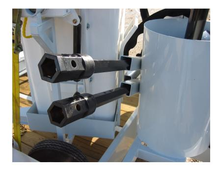
Before installing an extension bar to the auger bit, the bit must be disconnected from the driver motor. Two extension bars can be transported to the work site on the trailer.
