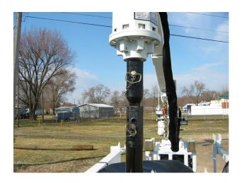
5. Slide extension into auger and pin it in place. Once the extension is in place, align the auger head above it and pin it to the extension.
