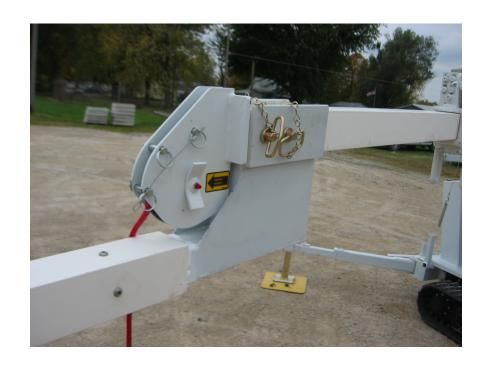
2. Pin bucket extension arm into the fiberglass 3<sup>rd</sup> stage boom.
