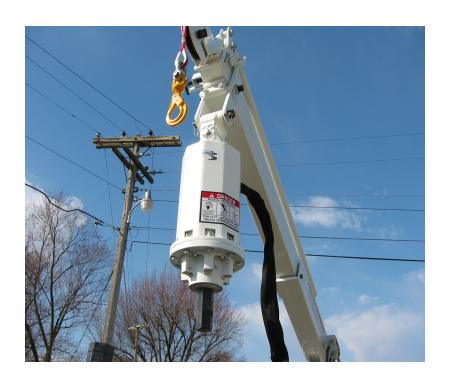
3. Carefully lift auger from the storage tubs.
