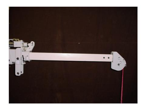
Manually extend the fiberglass boom extension fully (leaving the two hydraulic boom extensions retracted) and pin the last securable position. (DO NOT EXTEND HYDRAULIC STAGES.)
