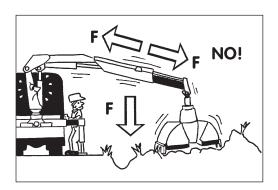
(!) WARNING (!) CRUSHING (F) OR PUSH (F) MANOEUVRES ARE NOT PERMITTED.
