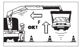
Do not rotate the crane before the load is lifted.
