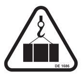
**DE 1686** Do not walk or stop under a suspended load
