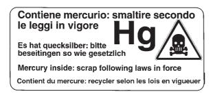
MERCURY IS EXTREMELY TOXIC. IN CASE OF REPLACEMENT AND/OR SCRAPPING, DISPOSE OF OR RECYCLE THE CAPSULE CONTAINING MER-CURY WITH MAXIMUM CARE, AND IN ACCORDANCE WITH THE NATIONAL REGULATIONS IN FORCE.
