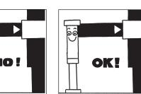
Remember that the stability of the unit (crane-vehicle) is only guaranteed by the complete lateral extension of the outriggers and by the observance of the capacity plates.
