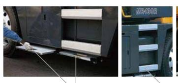
Aluminium step as standard equipment (600×600mm)
