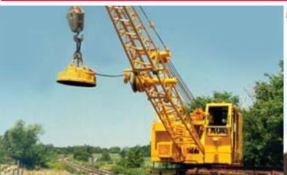
Rail dedicated 20 Ton Crane with 215 HP QSB Cummins Engine
