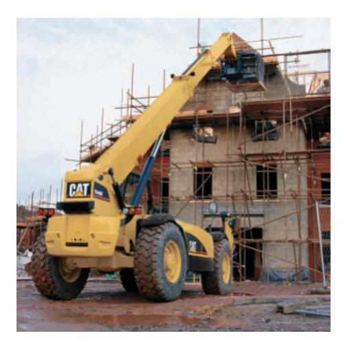
**Lift Height.** The TH460B can effectively and quickly place bricks, roofing materials and trusses to a maximum height of 44 ft (13.5 m).
