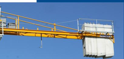
Ballast blocks: 2 types, 3 t and 1 t, allowing different ballasting combinations.
