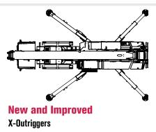
X-pattern outriggers are designed to offer maximum stability and strength.
