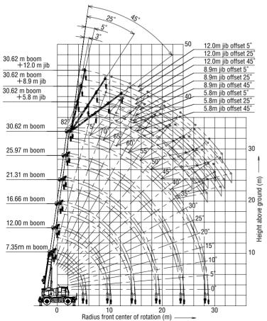
Boom and jib geometry shown does not reflect any deflection of boom and jib. Boom deflection and subsequent radius and boom angle change must be accounted for when at actual operation.
