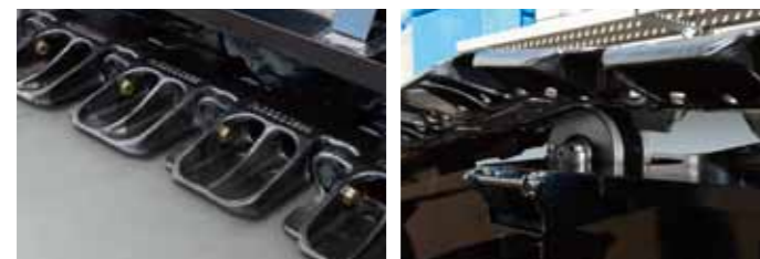
High-durability box type track shoes Lower rollers with 20% greater contact width
