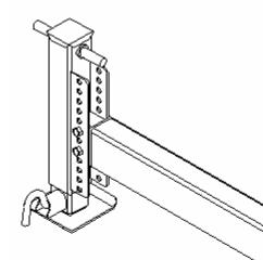
The Heavy Duty outriggers are designed for use with Liberator 4000 and larger cranes on trucks up to 33,000 GVW. For corner mounted cranes, they provide the maximum stability possible with your chassis by extending on the crane side only.
