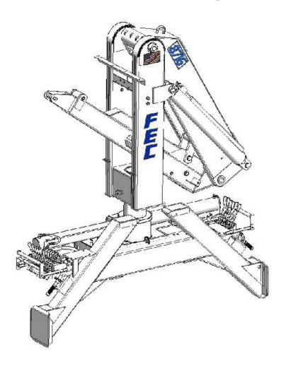
Load holding valves on all lift cylinders.
