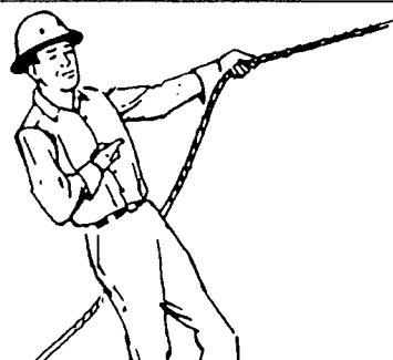
RETRACT BOOM (Telescoping Boom). One Hand Signal. One fist in front of chest, thumb pointing outward and heel of fist tapping chest.
