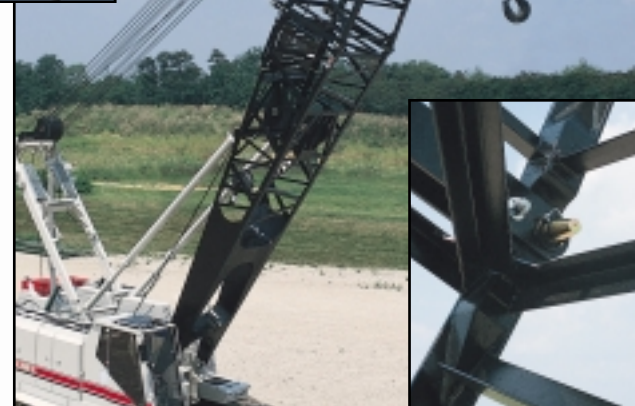
Seamless welds and treated hardware throughout attachment
