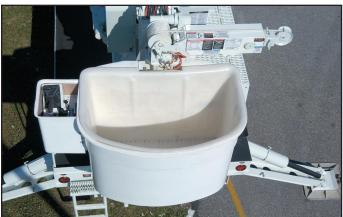
Hydraulically extendible jib may be manually rotated on its base and pinned in 5 working positions. Jib pinned perpendicular to upper boom (90°) is capable of lifting at maximum capacity, while located out of the way of operators.
