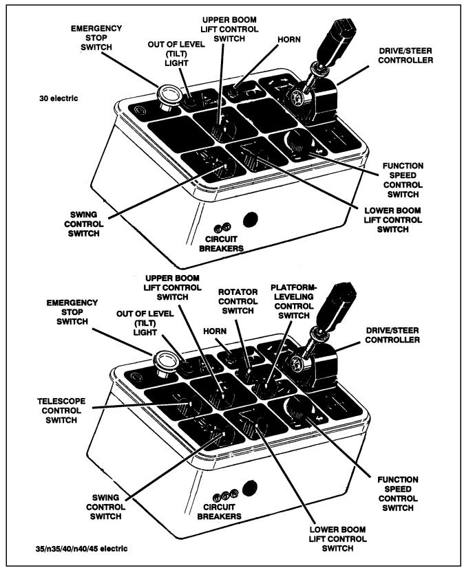
Figure 3-4. Platform Control Console.
