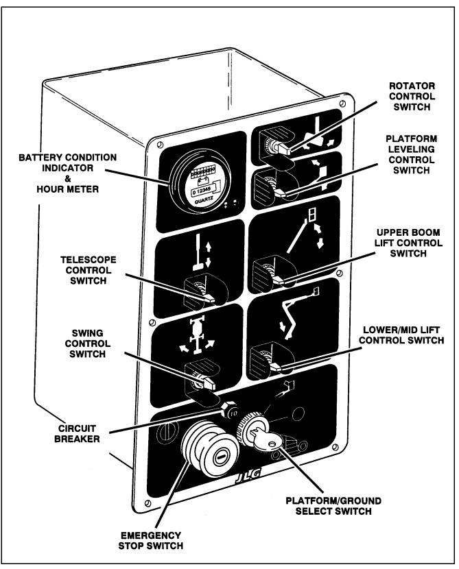
Figure 3-3. Ground Control Station, 35/n35/40/n40/45 electric. (Sheet 2 of 2)
