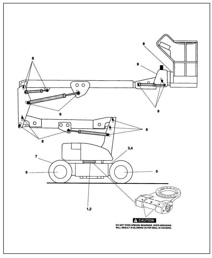
Figure 2-4. Lubrication Chart - 35/n35 electric. (Sheet 3 of 6)
