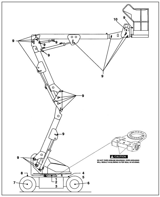
Figure 2-4. Lubrication Chart - 40/n40/45 electric. (Sheet 5 of 6)
