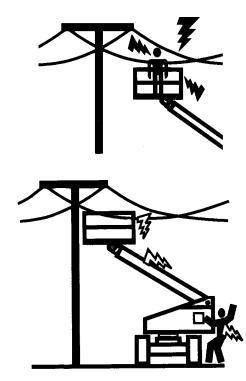
Maintain safe clearance from electrical lines, apparatus, or any energized (exposed or insulated) parts in accordance with the Minimum Safe Approach Distance (MSAD) as specified in Table 1-1. Allow for machine movement and electrical line swaying.
