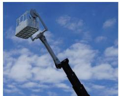
\* This extension is rated as non-insulated and not intended for energized work
