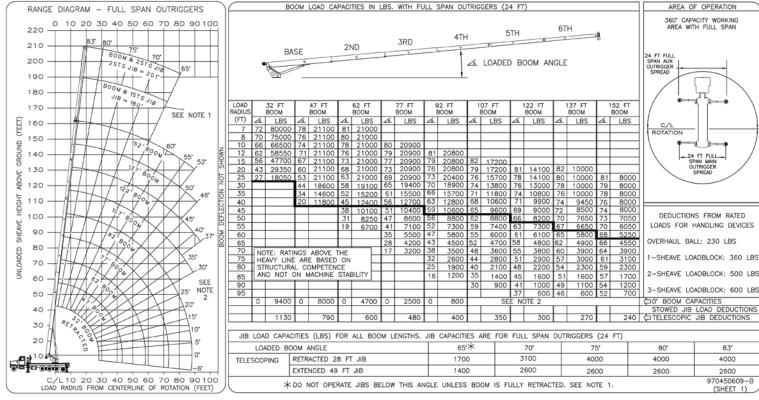
Note 1: When jib is erected, boom must be fully retracted before lowering below minimum boom with jib angles. Retracted boom with jib has no lifting capacity below a 50 degree angle with full span outriggers and below a 65 degree angle not shown on jib load rating chart.
