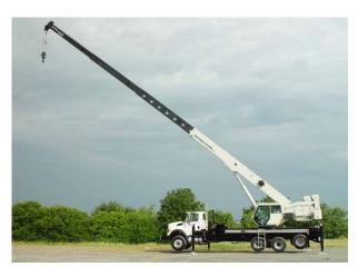
**Four or five-section boom** The Series NBT50 can be equipped with two different boom lengths 31,1 m (102 ft) and 39,01 m (128 ft).
