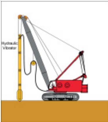
Deep Compaction Vibrator
