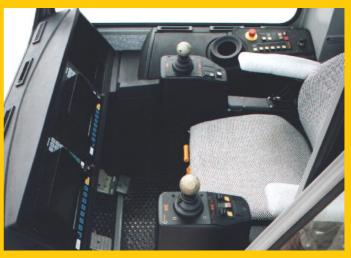
State of the art control and display systems for a save crane operation.
