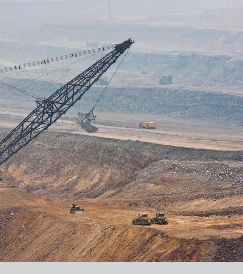
Delivering extremely high levels of overburden removal productivity at a low cost per tonne (ton), the Cat 8200 model dragline offers all of the innovative technology of our flagship model – the Cat 8750 – but on a mid-range size scale. Along with a lower initial capital outlay compared to larger draglines, the 8200's unique combination of technology, size, and long operating life ensures the low total cost of ownership you need for a strong return on your investment.
