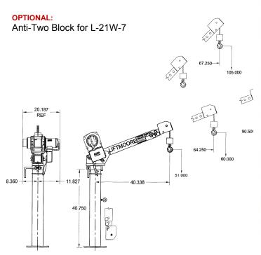
Boom telescopes from 3' 3" to 7' 3"
