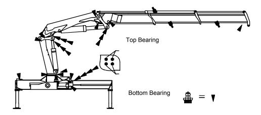
Example of a lubrication chart. For specific loader model, please see lubrication label on loader/Fly-Jib.
