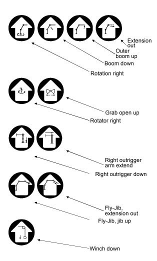
Each control valve has a label showing the functions of that particular valve.
