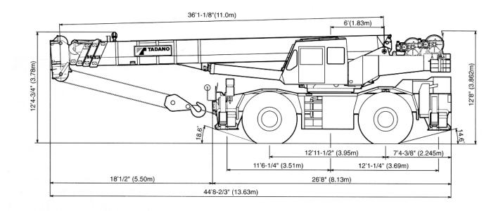
Note: Dimension is with boom angle at  $-1.5^{\circ}$ .
