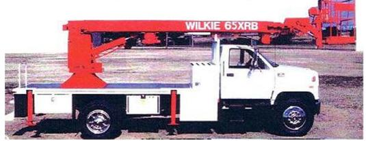
TOTAL HYDRAULIC JOYSTICK BASKET CONTROLS PROPORTIONAL BASE CONTROLS 5000# LIFT WINCH 400# JIB WINCH ROTATING BASKET POWER LEVELED BASKET
