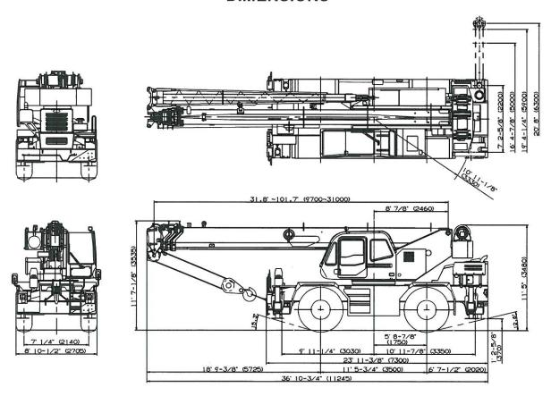
Note: Dimension is with boom angle at 0 degree.
