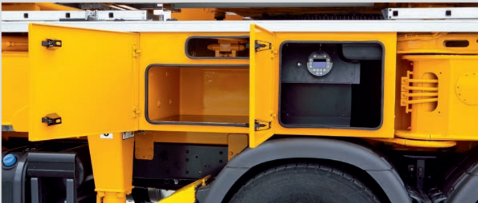
Extensive storage boxes for equipment and support timber are provided at the intermediate frame and the two front folding beams
