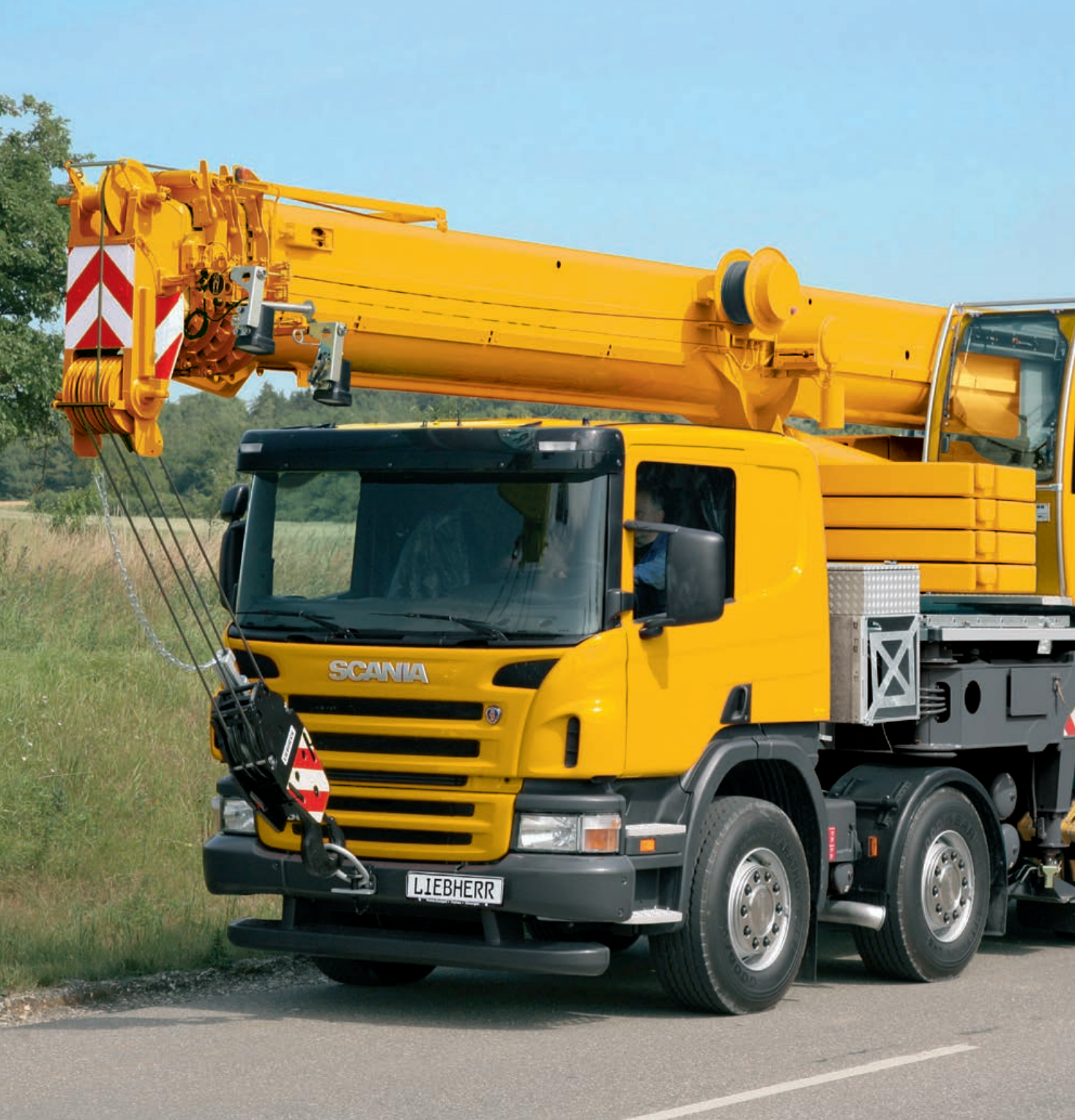
Extensive storage boxes for equipment and support timber are provided at the intermediate frame and the two front folding beams
